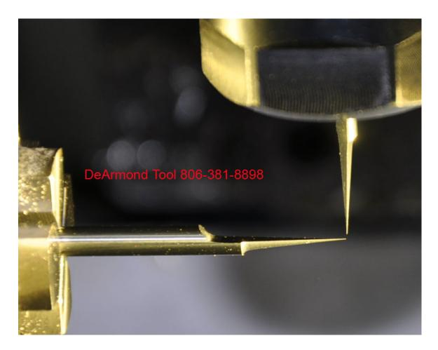
!! NOTE: MAKE SURE after setting the tool that FROM "Z" -0, that you have room in "Z" for a minimum of 50 mm positive "Z" movement! After cutting one side, the rotary AUTOMATICALLY rotates & the program cuts the back side of the model. During this rotation... the "Z" axis moves the tool tip up 50 mm from "Z"-0.
